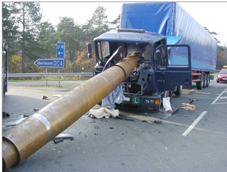
Figure (Ridder): Seventeen tonnes of steel pipes inserted inside one another. Simply a braking maneuver, i.e. normal acceleration.
