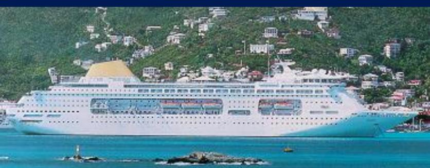
... side recesses for lifeboat stowage give a complex structural response ...
