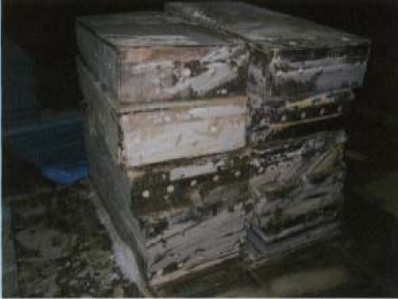
Resulting primary and secondary insulation boxes soaked in seawater
