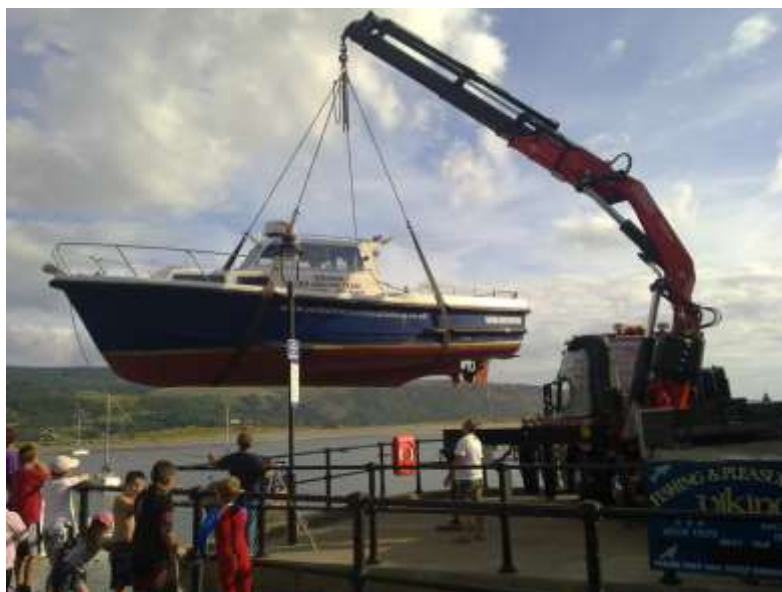
Figure 10 - failing to use spreaders resulting in crush damage
