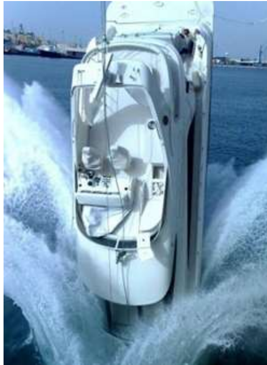
Figure 9 - consequences of lifting band slippage
