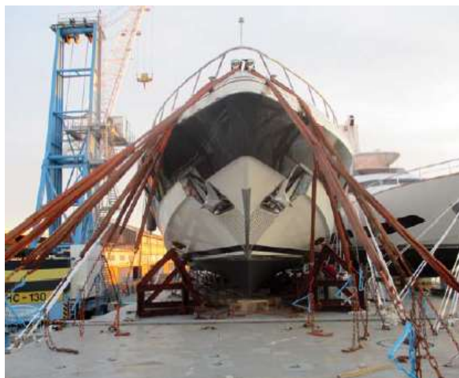
Figure 4 - excessive use of inappropriate fixture
