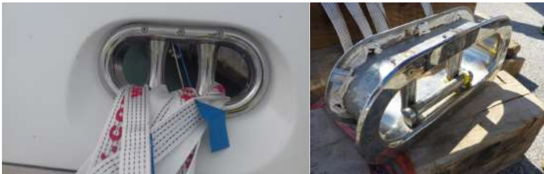
Figure 6 - consequences of using inappropriate fixtures, before and after
