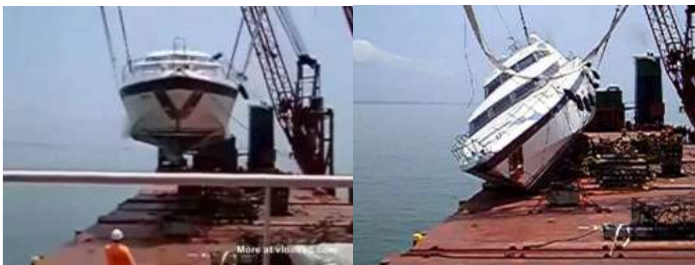
Figure 8 - gear failure causes yacht to fall
