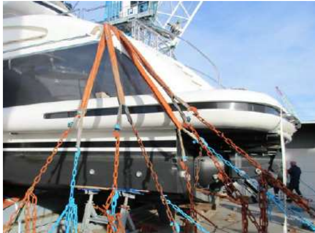
Figure 5 - excessive use of fixture and a source of damage to gel coat
