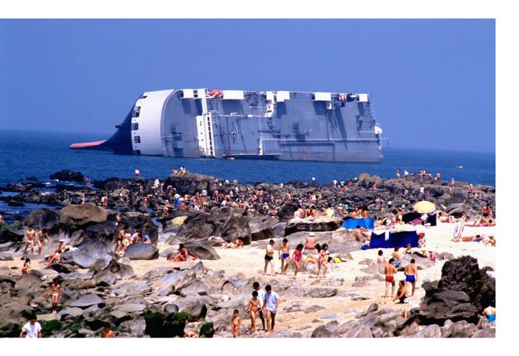
Inadequate stability on departure, open pilot door
