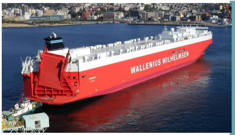
High sides vessels with relatively light draught. NB Offset stern door and ramp
