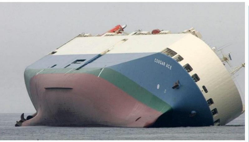
Angle of loll during ballast water exchange.
