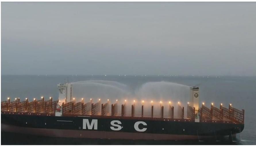
Active fire fighting on deck: water curtains, water screens, fixed water monitors
