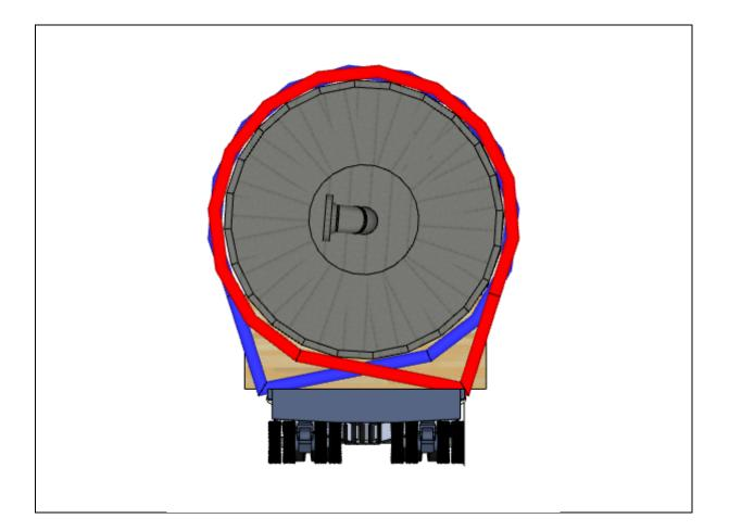
The red loop does not secure the cargo against movement to the left because to do so, both ends of the belt would have to be pulled in the same direction (see above illustration of the column secured in the vessel). As this sketch shows, however, the right end of the belt is directed to the right side (as seen from the attachment point of the lashing) and thus loses its retention force.
