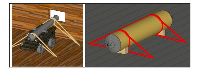
The vertical loop lashing is known internationally as the C-loop. The C-loop generally works well when the cargo is narrower than the means of transport to which the lashings are attached.
