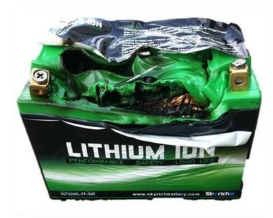
Mechanical abuse of the battery from drops, impacts, abrasion, vibration
