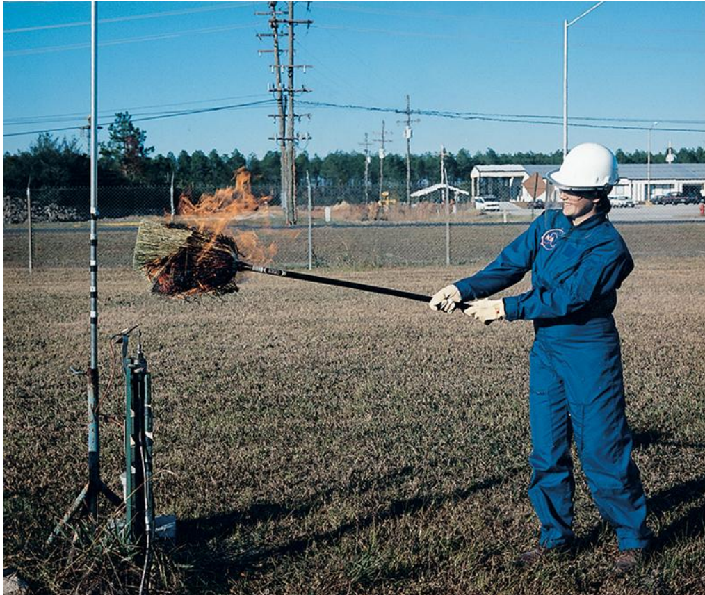
NASA engineer Heidi Barnes demonstrates the antiquated "broom method" of detecting invisible hydrogen and alcohol fires (Credit : NASA)
